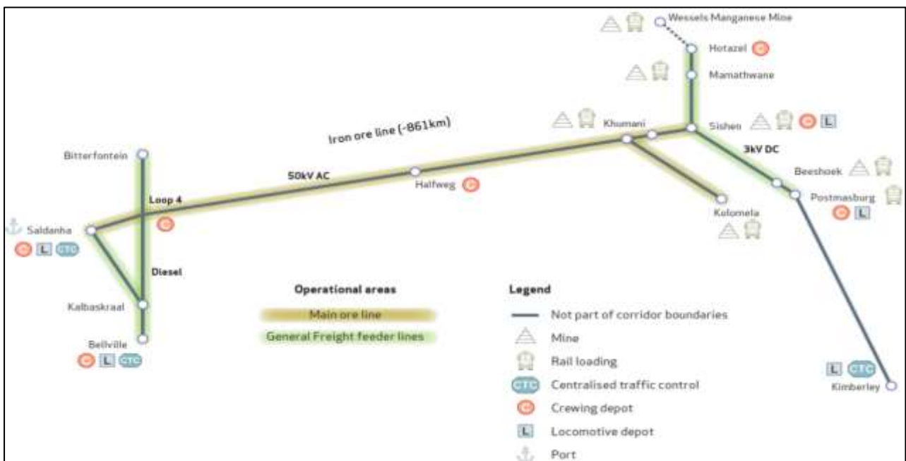
Figure 9: Ore corridor key lines (Source: Transnet)
